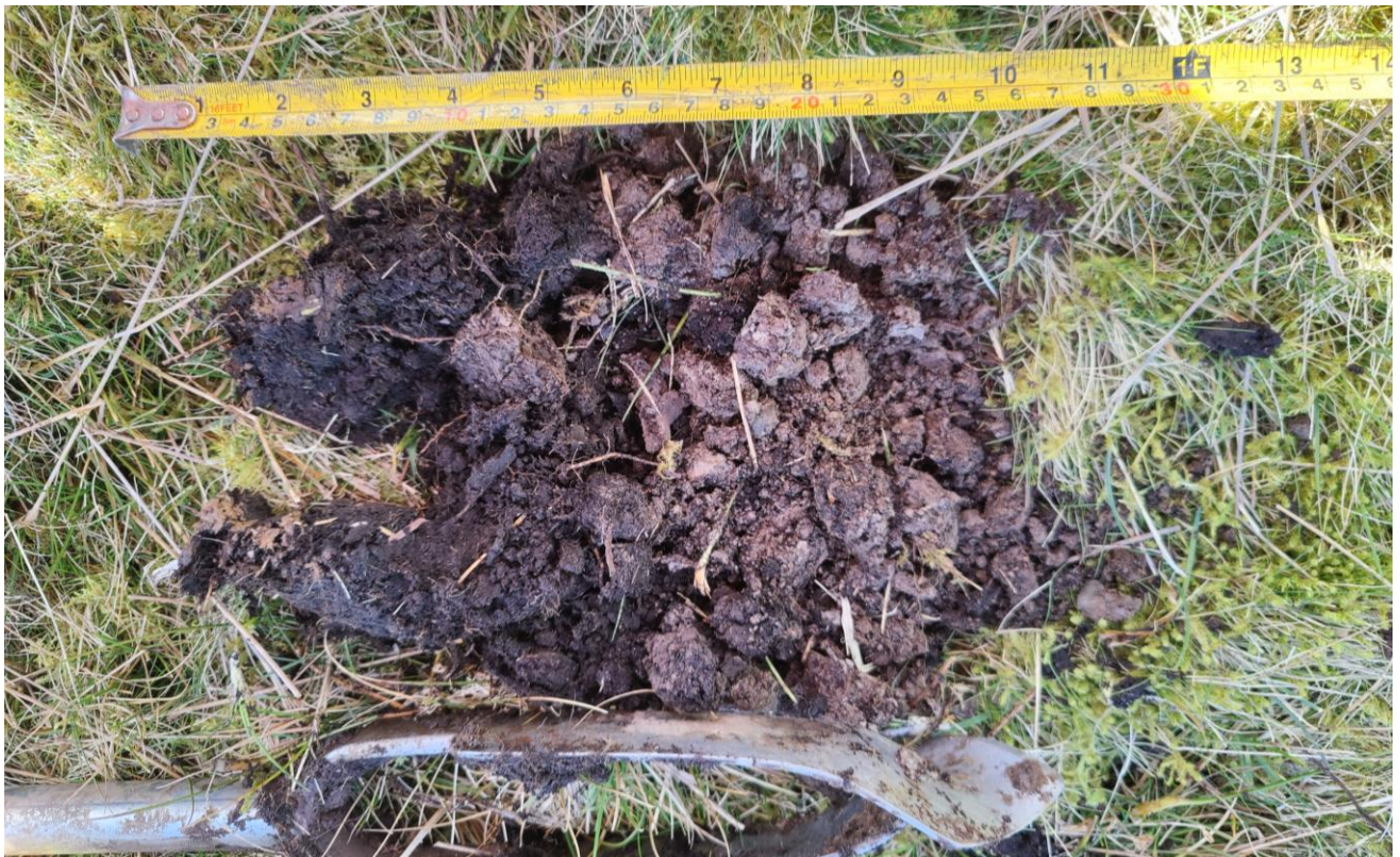
Plate 10A-4 – Peaty profile at T08. The core illustrates dark brownish, black very fibrous, slightly clayey peat – H2, B1, F2/3, C0, W0 at ~ 0.13 m but becomes light grey, occasionally darker grey / brown gravelly, silty clay at ~ 0.2 m. The gravel is subangular fine and medium tabular rough of sandstone. NGR: SN 99858 98776.
