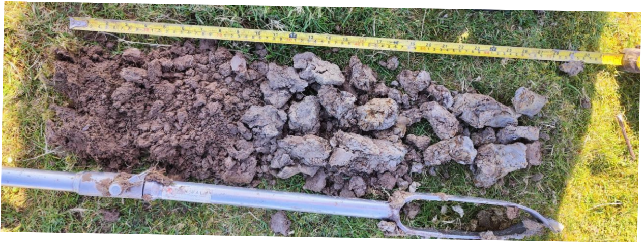
Plate 10A-3 – Clay profile at T02 with soft dark greyish, brown clay with slight rootlets, becoming firm, pale grey clay with light reddish orange and light reddish brown mottles and a slight inclusion of rootlets. NGR: SO 00903 97850.
